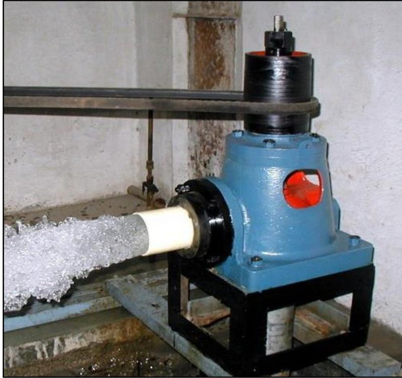
Gambar 3.20. Pompa Turbine
